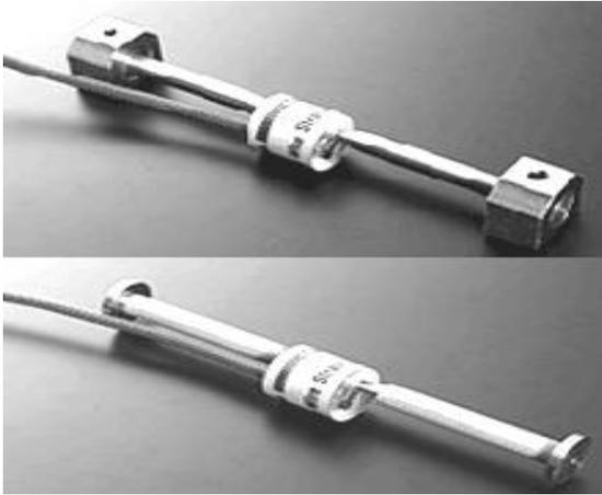
Systel Series 1000 model Strain Gage is designed to measure the changes in strain in and on structural members associated with many types of structure.
